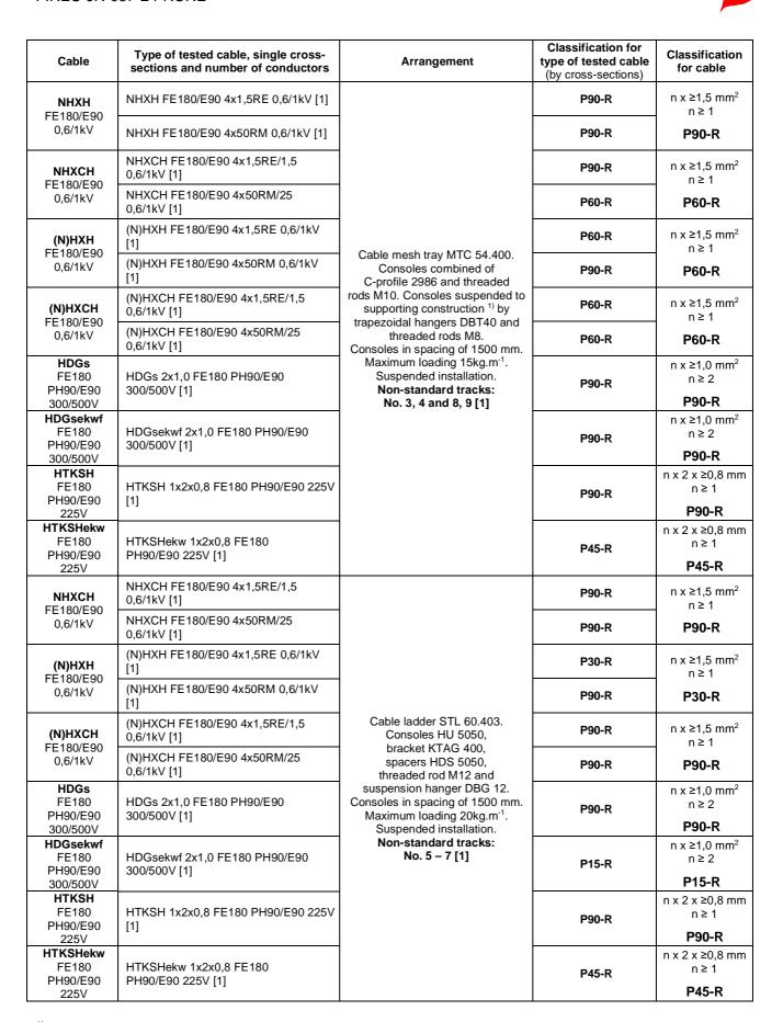
Supporting construction is made of segments of steel sheets 1,2 mm thick bent to wave 550 mm long. Individual segments are fixed to ceiling by 4 pcs of anchors in spacing of 1500 mm.
