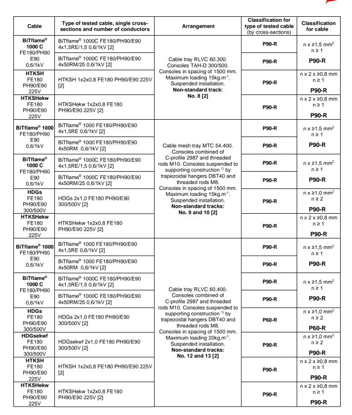
1) Supporting construction is made of segments of steel sheets 1,2 mm thick bent to wave 550 mm long. Individual segments are fixed to ceiling by 4 pcs of anchors in spacing of 1500 mm.
